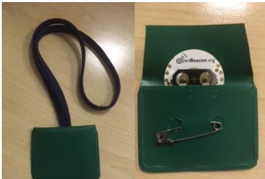
Figure 2: Packaging of proximity sensor
