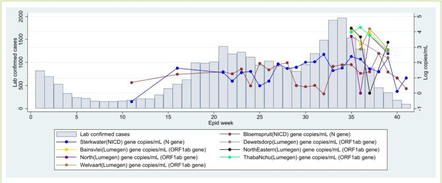
**Figure 3.** Laboratory confirmed cases of SARS-CoV-2 (bars) and levels of SARS-CoV-2 in log copies/mL of wastewater (coloured lines) from wastewater treatment plants (WWTPs) in Mangaung, Free State Province during epidemiological weeks 1-41, 2021. The testing laboratory and quantified SARS-CoV-2 gene is named in brackets after the name of the WWTP. Note that comparisons of levels over time should only be done for specimens tested in the same laboratory
