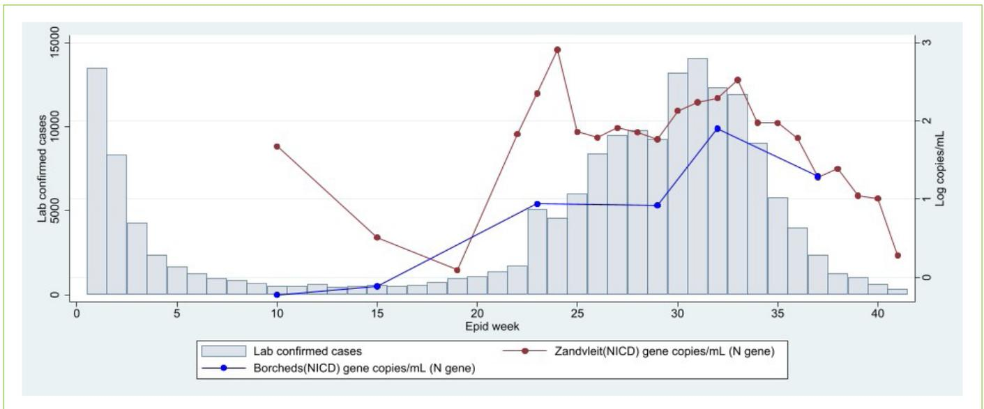
**Figure 5.** Laboratory confirmed cases of SARS-CoV-2 (bars) and levels of SARS-CoV-2 in log copies/ml of wastewater (coloured lines) from wastewater treatment plants (WWTPs) in City of Cape Town, Western Cape Province during epidemiological weeks 1-41, 2021. The testing laboratory and quantified SARS-CoV-2 gene is named in brackets after the name of the WWTP.
