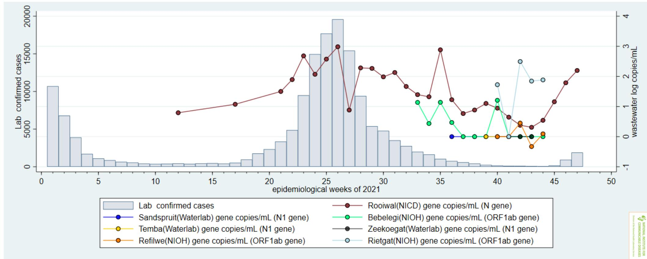
Changes in SARS-CoV-2 viral load (data points and coloured lines) in in-flowing untreated wastewater from plants in City of Tshwane, compared with laboratory-confirmed cases resident in City of Tshwane (grey bars), by epidemiological week, 2021
