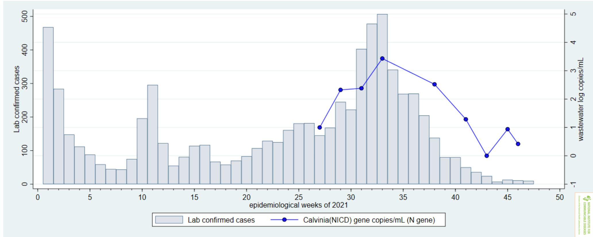
Changes in SARS-CoV-2 viral load (data points and coloured lines) in in-flowing untreated wastewater from a plant in the Northern Cape Province, compared with laboratory-confirmed cases resident in Namakwa (grey bars), by epidemiological week, 2021
