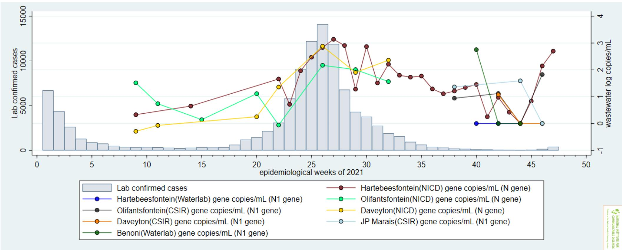
Changes in SARS-CoV-2 viral load (data points and coloured lines) in in-flowing untreated wastewater from plants in Ekurhuleni, compared with laboratory-confirmed cases resident in Ekurhuleni (grey bars), by epidemiological week, 2021
