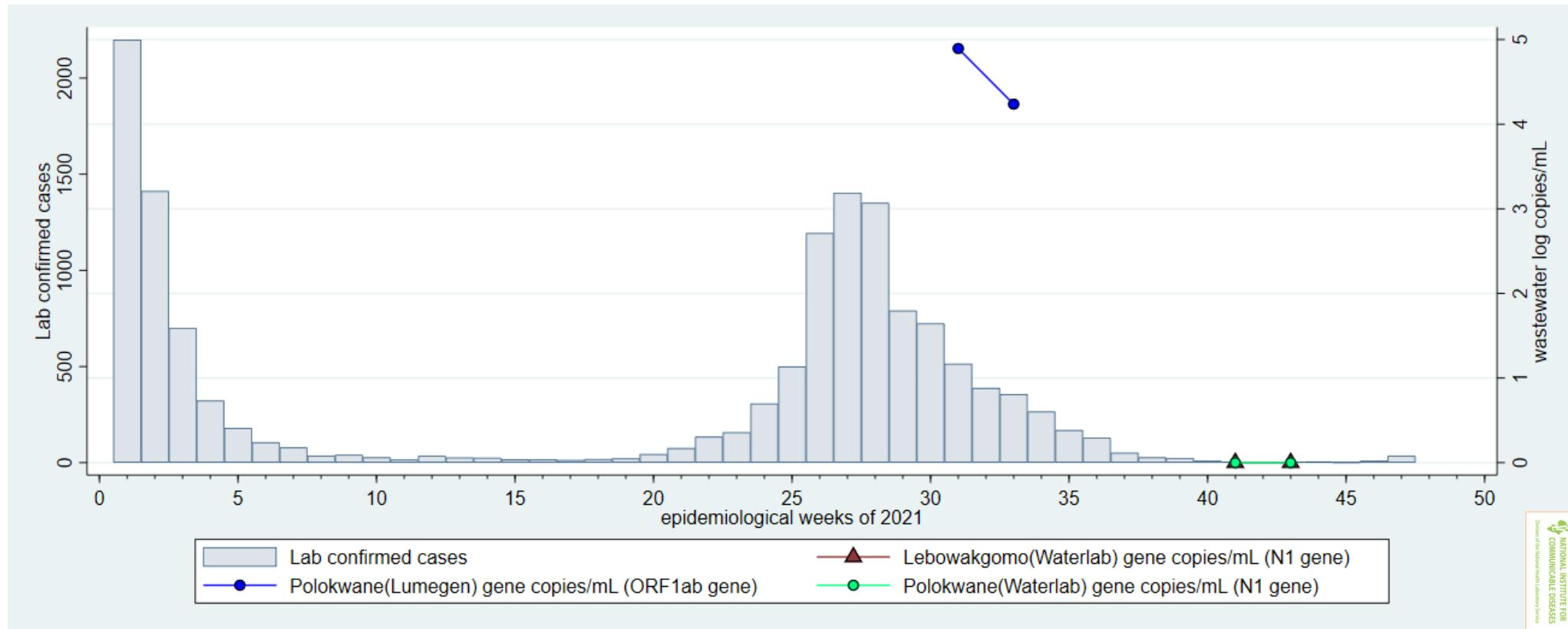
Changes in SARS-CoV-2 viral load (data points and coloured lines) in in-flowing untreated wastewater from a plant in the Limpopo Province, compared with laboratory-confirmed cases resident in Polokwane (grey bars), by epidemiological week, 2021
