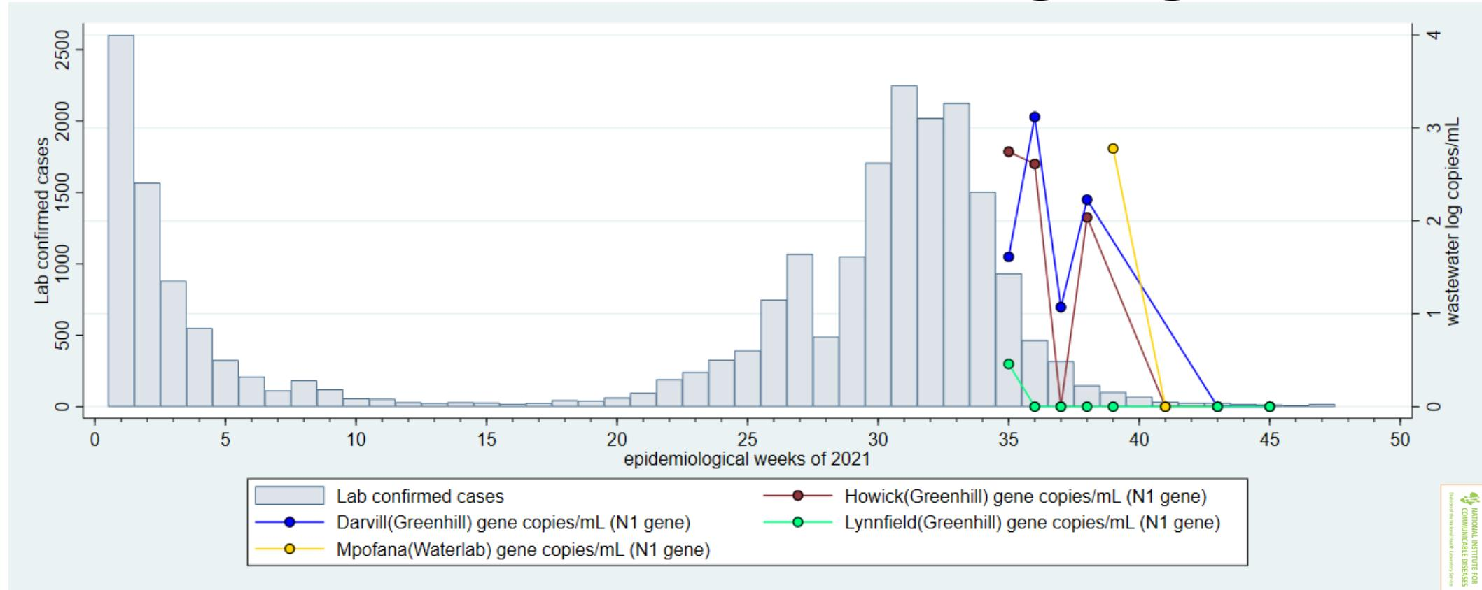
Changes in SARS-CoV-2 viral load (data points and coloured lines) in in-flowing untreated wastewater from plants in Mgungundlovu, compared with laboratory-confirmed cases resident in Umgungundlovu (grey bars), by epidemiological week, 2021
