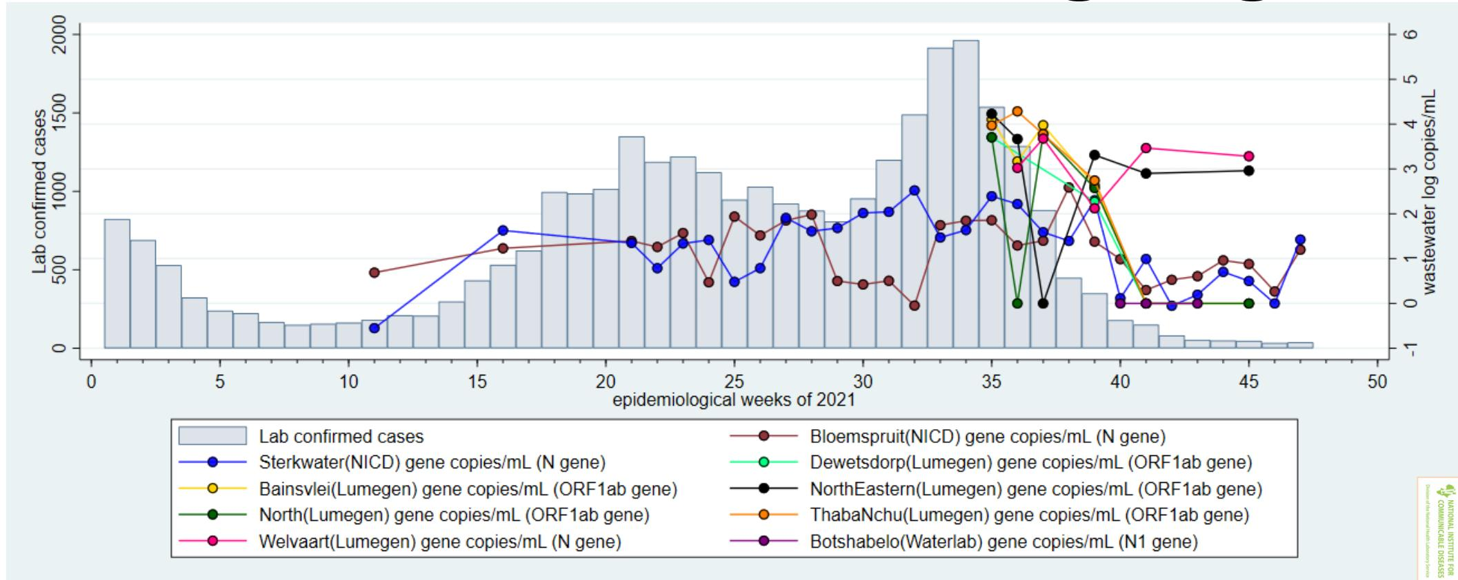
Changes in SARS-CoV-2 viral load (data points and coloured lines) in in-flowing untreated wastewater from plants in Mangaung, compared with laboratory-confirmed cases in Mangaung (grey bars), by epidemiological week, 2021
